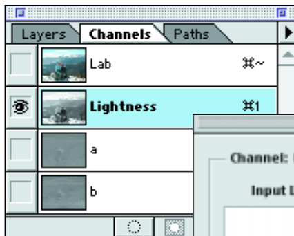
Figure 2: When the Lightness channel in the Channels palette is highlighted, the image turns to grayscale. By adjusting brightness and contrast here, we can affect the perceived sharpness of the image.
